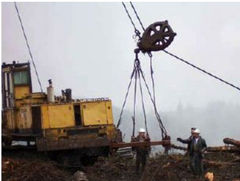
The Berger tower yarder has a solid reputation for working ecologically sensitive areas. It was used in the high profile restoration work at Mt. St. Helens.
