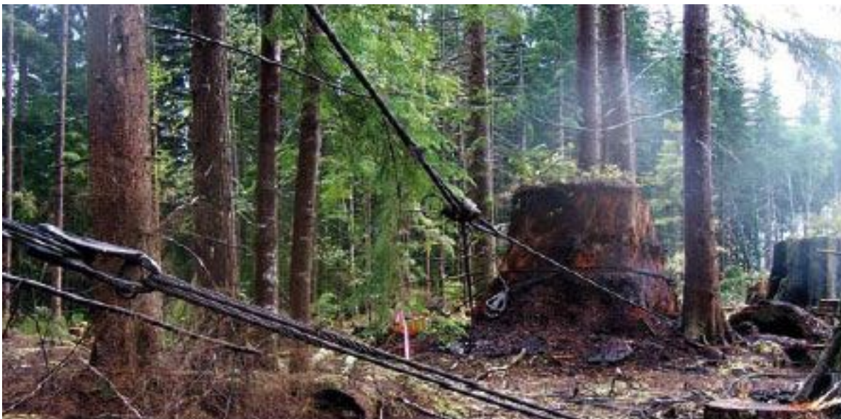
A large old growth stump was used as the tail tree. It measured approximately 42 feet around.
