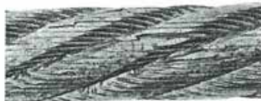
5. Severe wear, associated with high tread pressure. Protrusion of fibre main core.
