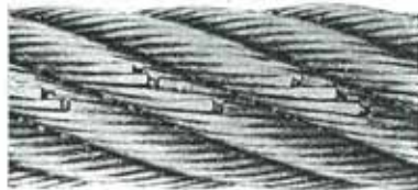
3. Narrow path of wear resulting in fatigue fractures, caused by working in a grossly oversize groove, or over small support rollers.
