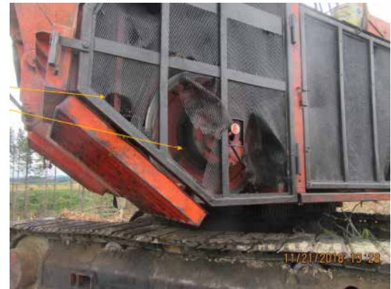
Damaged mesh guard over rotating parts. Access by skilled personnel may be required for maintenance with parts rotating. A risk assessment should be undertaken to decide if interlocking or other measures are required.
