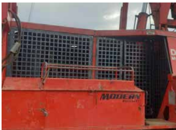
Comprehensively guarded engine compartment. Again, depending on the risks, interlocking may be required.
