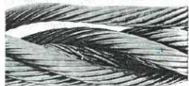
11. Break up of IWRC resulting from high stress application. Note nicking of wires in outer strands.
