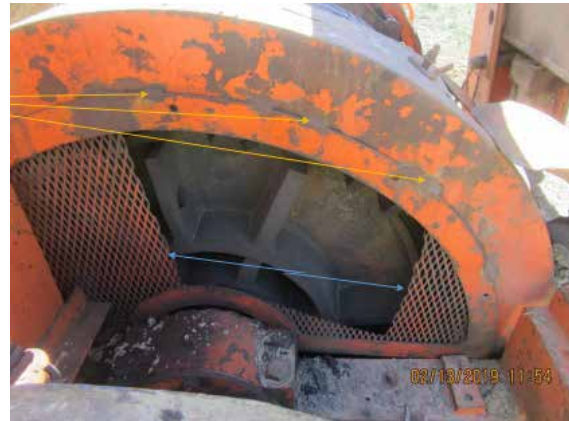
OEM guard (missing) had been replaced with the welded mesh shown after a toe amputation. Guard was not removable "using tools", so has been cut out at some time to attach a new skyline.
