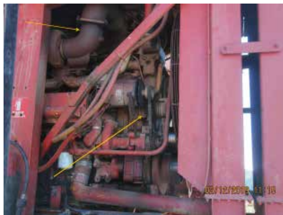
Entanglement risk from exposed belts and pulleys.
