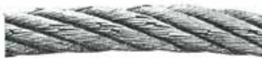
4. Two parallel paths of broken wires indicative of bending through an undersize groove in the sheave.
