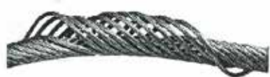
14. Multi strand rope 'bird caged' due to torsional unbalance. Typical of build up seen at anchorage end of multi-fall crane application.
